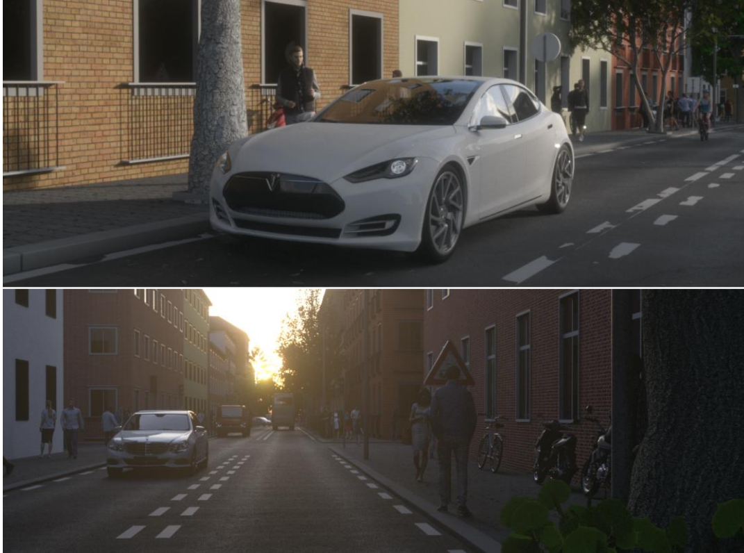
Figure 3. Two images generated using our computer graphics system simulating the cameras on a self driving car. As shown in Figure 2, we generate both the camera image and the corresponding ground truth information required to train the machine learning system to learn semantic segmentation and identify what is what in the input image.
