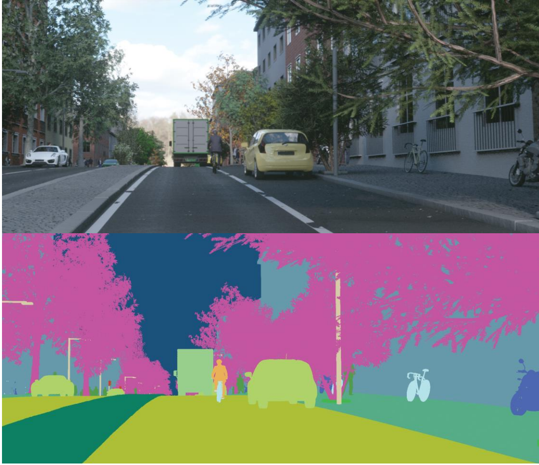
Figure 2. A semantic segmentation algorithm can identify which part of an input image (top) belongs to a specific class such as car, pedestrian, road, building etc. The segmentation map (bottom) shows the extent of the different classes captured in the images. This also demonstrates the visual fidelity of the synthetic data as the input images are generated using photo-realistic image synthesis.
